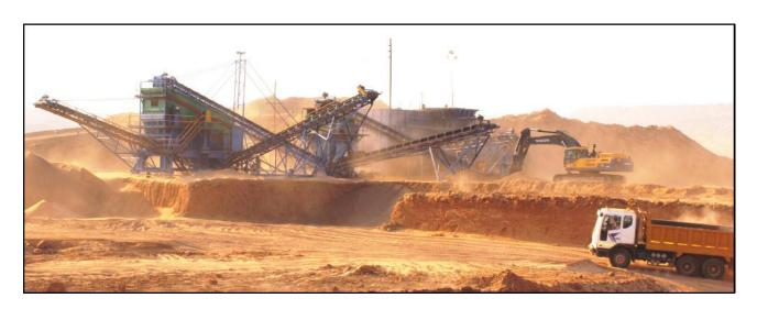
Figure 18-6 In-field Dry Screening Plant and Trommel
