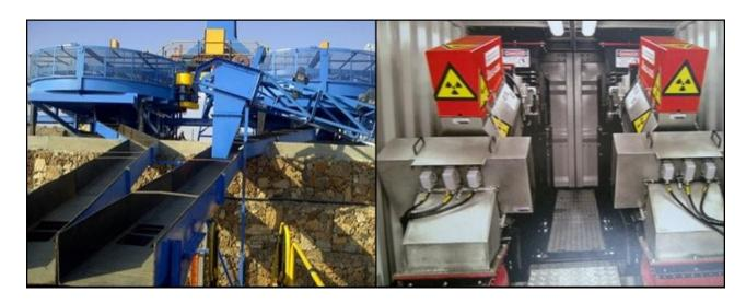
Figure 18-9 Rotary Pans and X-ray FlowSort Final Recovery
