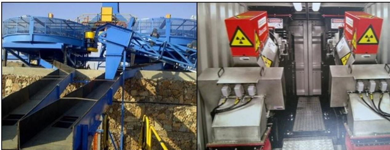
**Figure 18-9 Rotary Pans and X-ray FlowSort Final Recovery**
