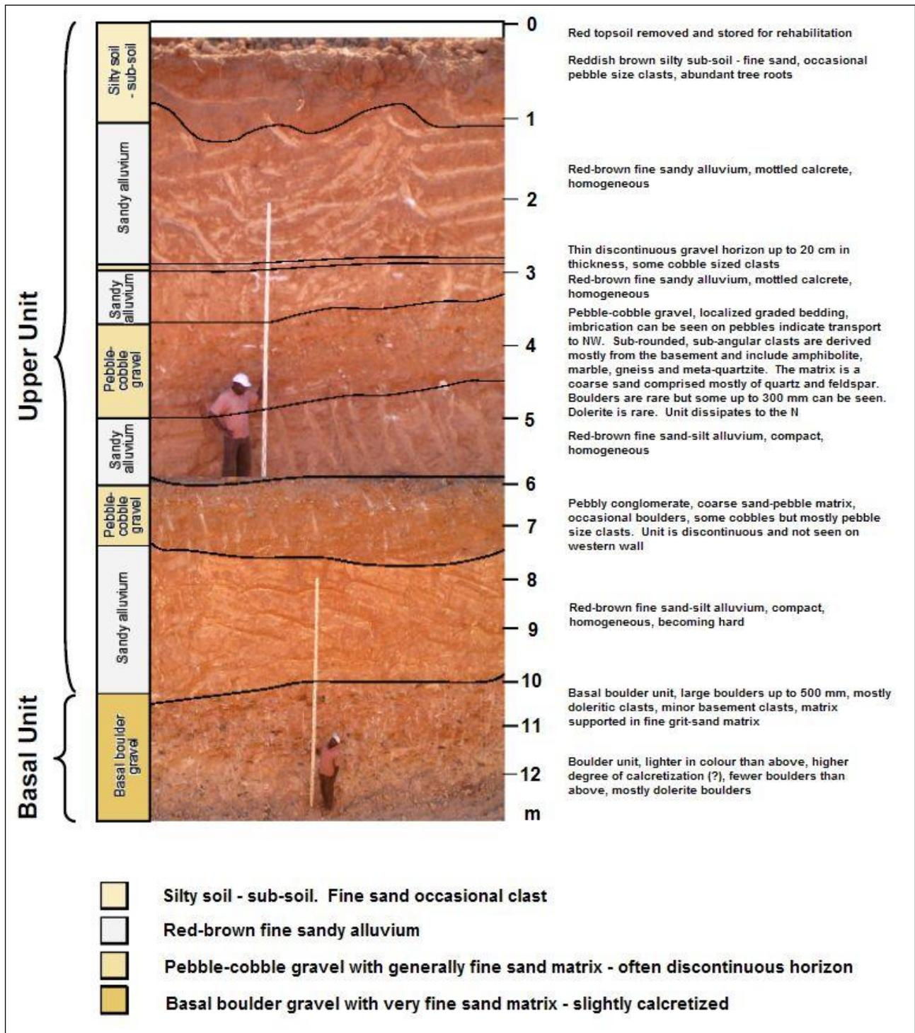
**Figure 7-3 The Stratigraphy of the Krone-Endora Deposit, as visible in the northeast wall of Pit 1 of the 2004 sampling programme (after Spooner, 2004 and Millad, 2005)**
