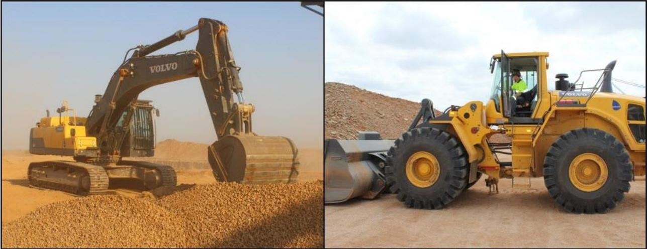
**Figure 18-11 Excavator and Front-End Loader**
