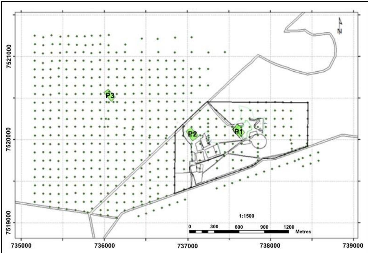
**Figure 10-2 RC Drilling positions on the Krone-Endora Project**
