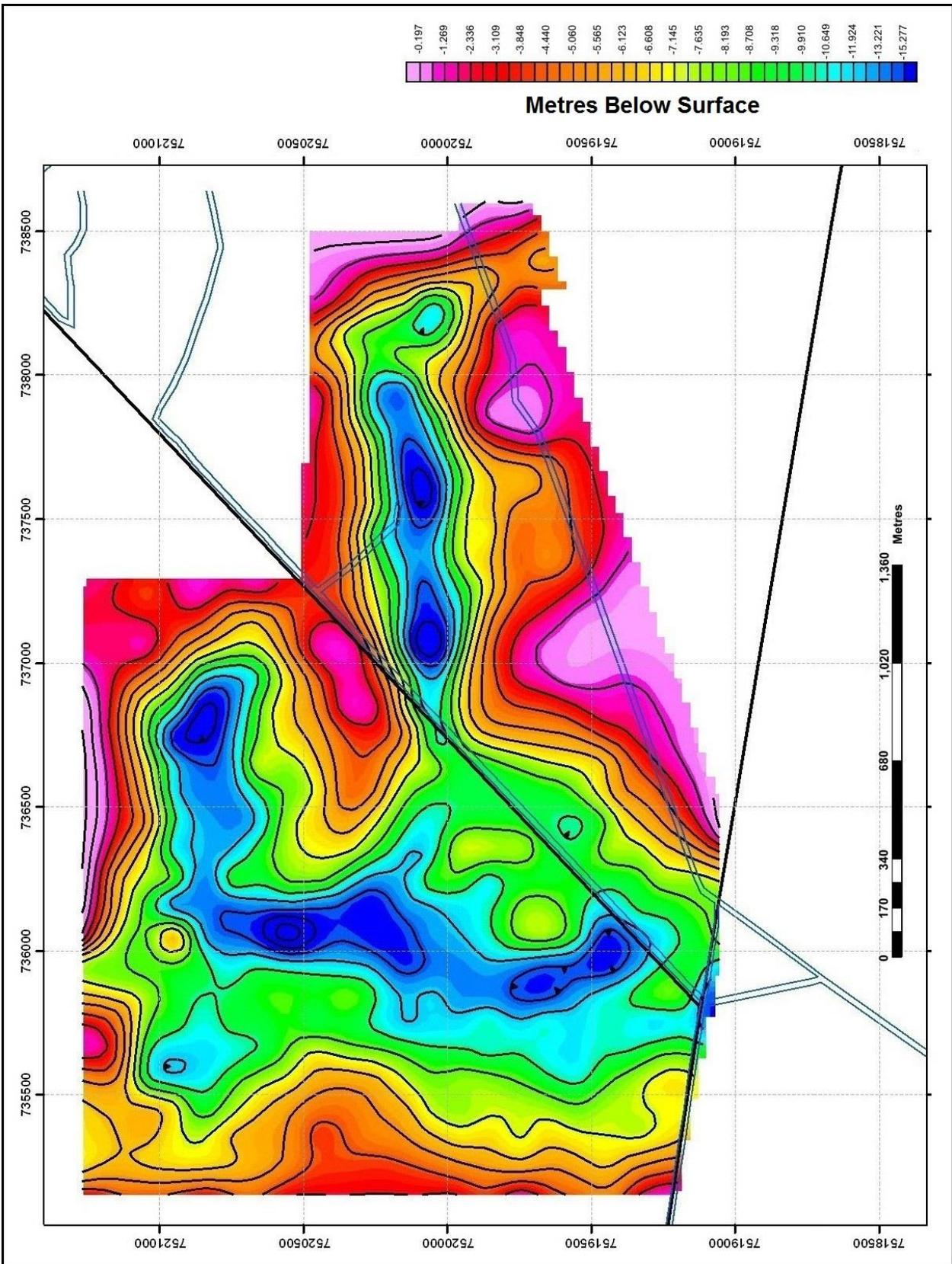
**Figure 10-3 Bedrock Topography Map, based on RC drilling**
