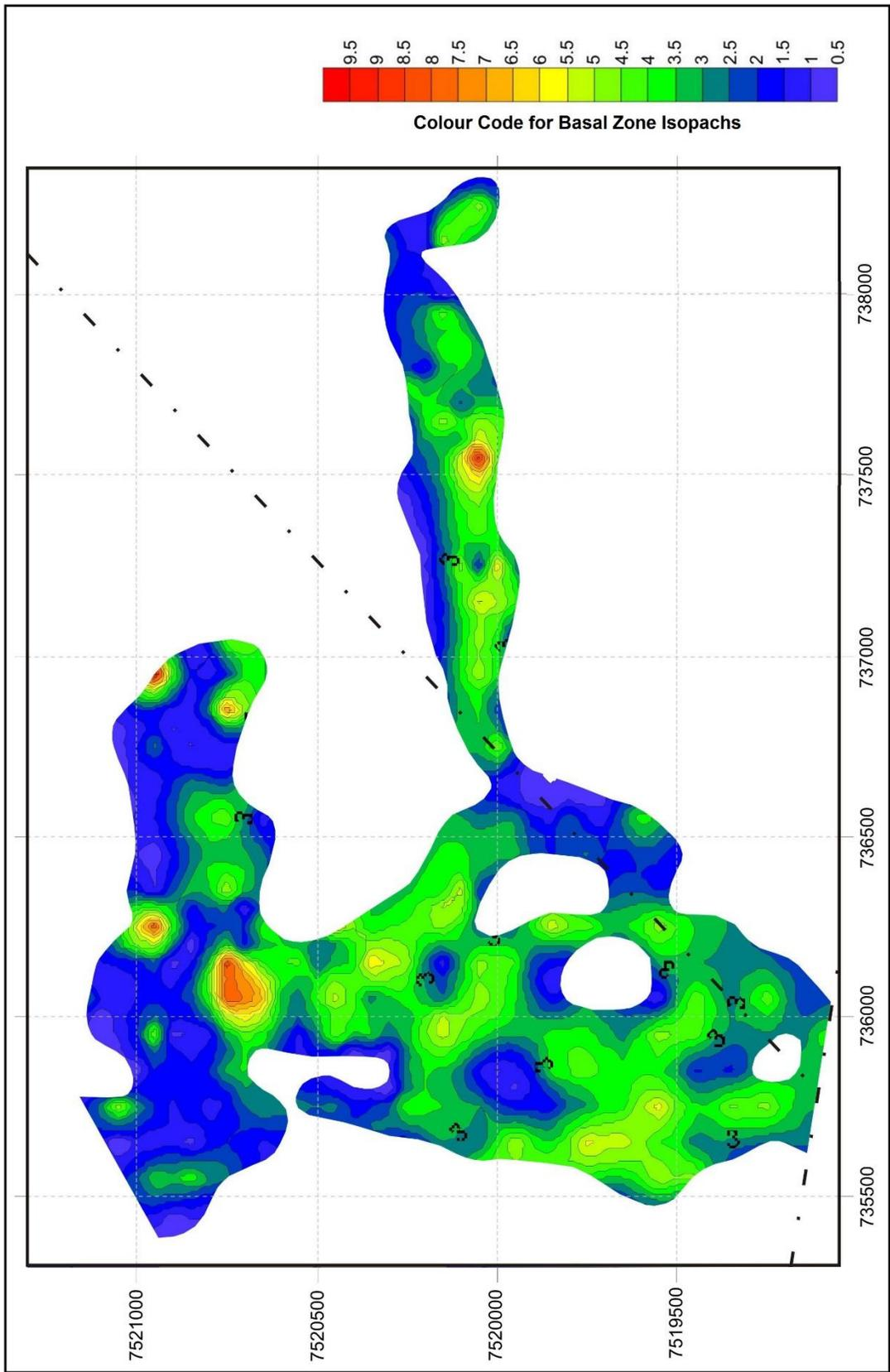
**Figure 10-5 Basal Gravels Thickness Isopach, based on RC drilling**
