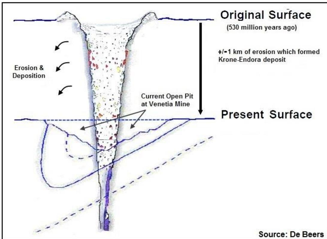
**Figure 8-1 Proposed Erosion of the Venetia K1 Kimberlite Pipe**
