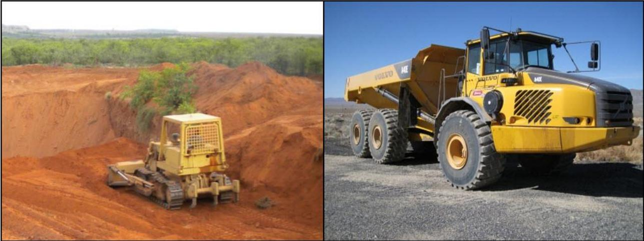
**Figure 18-12 Bulldozer and Articulated Dump Truck**
