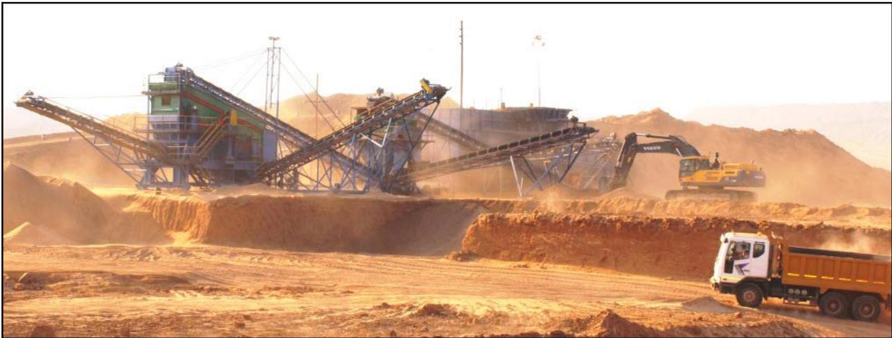
**Figure 18-6 In-field Dry Screening Plant and Trommel**
