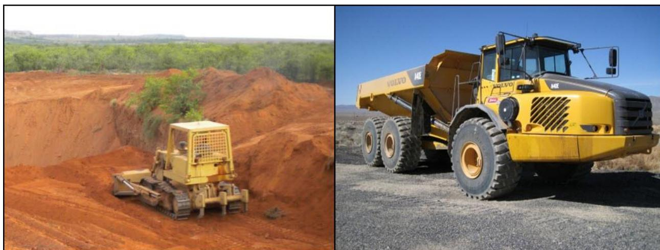
**Figure 18-12 Bulldozer and Articulated Dump Truck**
