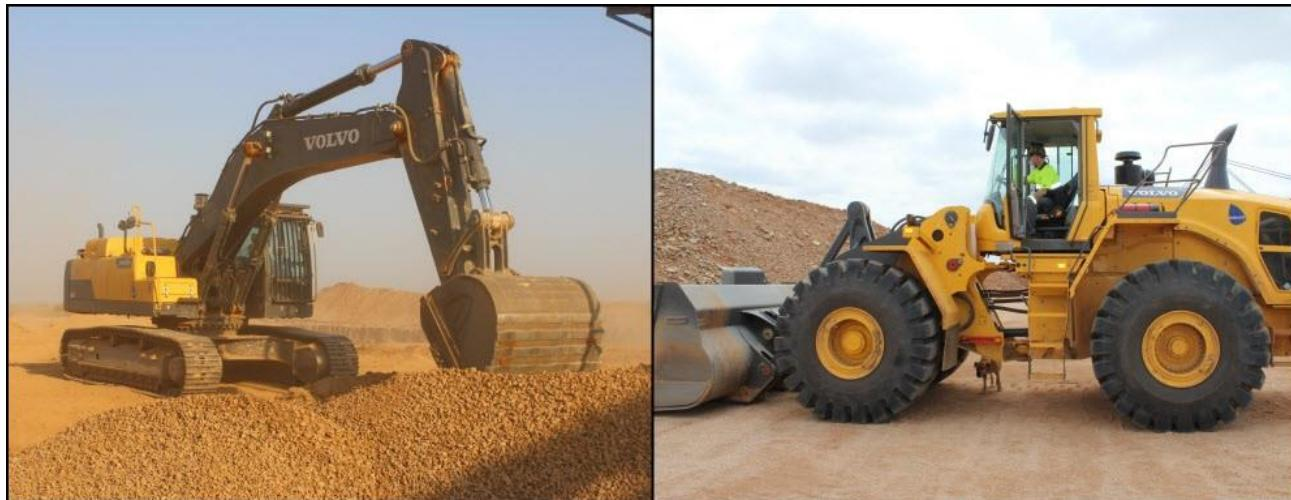
**Figure 18-11 Excavator and Front-End Loader**
