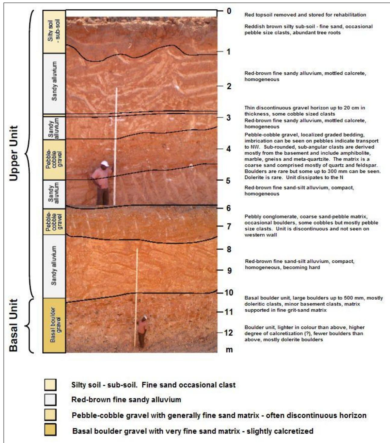
**Figure 7-3 The Stratigraphy of the Krone-Endora Deposit, as visible in the northeast wall of Pit 1 of the 2004 sampling programme (after Spooner, 2004 and Millad, 2005)**
